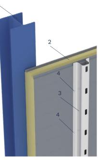
Figure 2. Transversal fixing of suspended facade mounting profiles: 1: support structure; 2: wall panel; 3: suspended facade mounting profile; 4: screw/rivet
