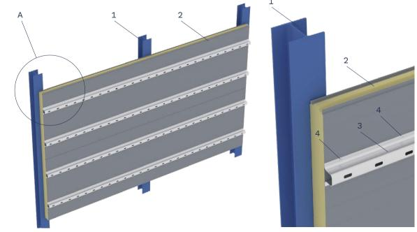
Figure 1. Longitudinal fixing of suspended facade mounting profiles: 1: support structure; 2: wall panel; 3: suspended facade mounting profile; 4: screw/rivet
