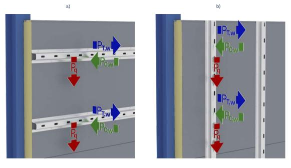
Figure 3. Loads created by the suspended facade:  $P_q$ : transversal force created by the self weight of a suspended facade;  $P_{T,w}$ : tensile load created by the wind load;  $P_{c,w}$ : compression force created by the wind load; a) mounting profiles fixed longitudinally to the panel; b) mounting profiles fixed transversally to the panel.
