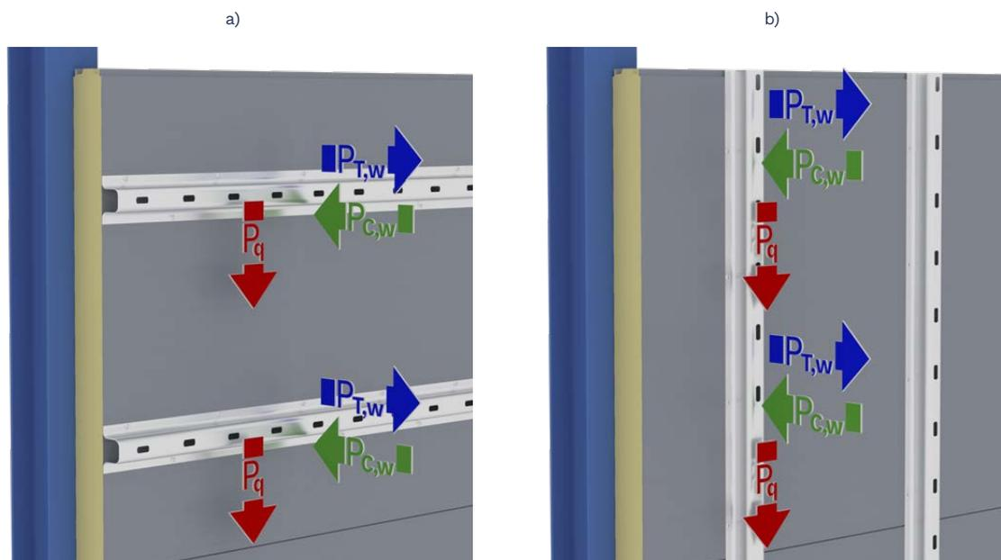
Figure 3. Loads created by the suspended facade:  $P_q$ : transversal force created by the self weight of a suspended facade;  $P_{T,w}$ : tensile load created by the wind load;  $P_{C,w}$ : compression force created by the wind load; a) mounting profiles fixed longitudinally to the panel; b) mounting profiles fixed transversally to the panel.
