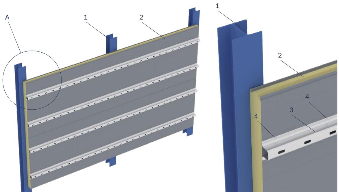
Figure 1. Longitudinal fixing of suspended facade mounting profiles:
