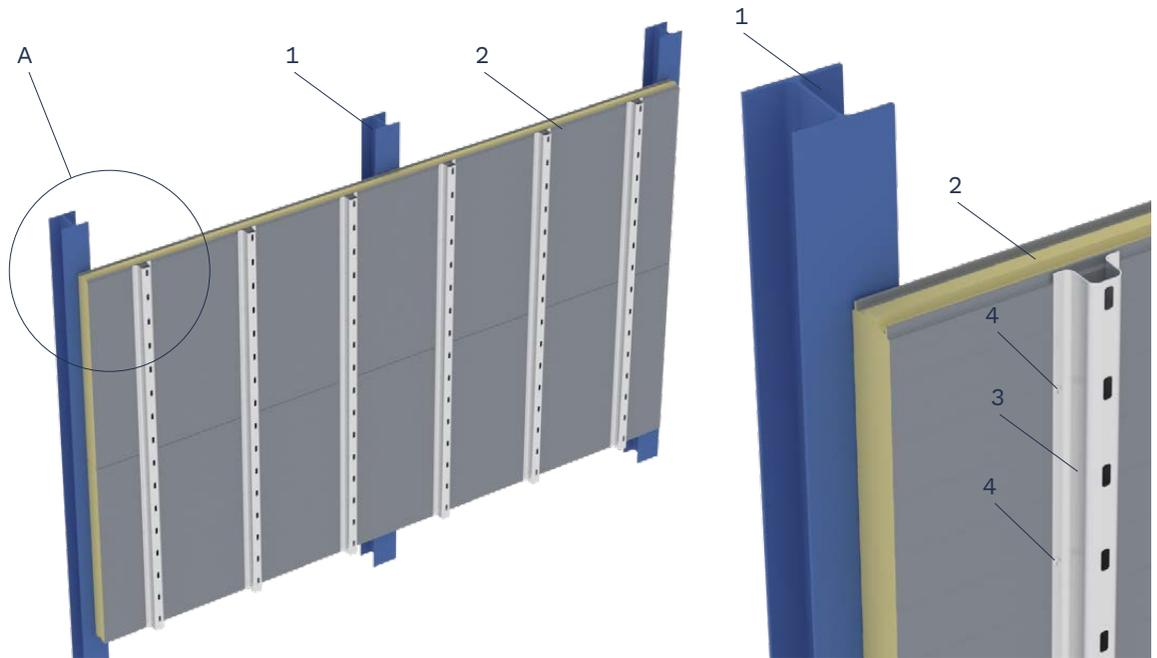
Figure 2. Transversal fixing of suspended facade mounting profiles:
